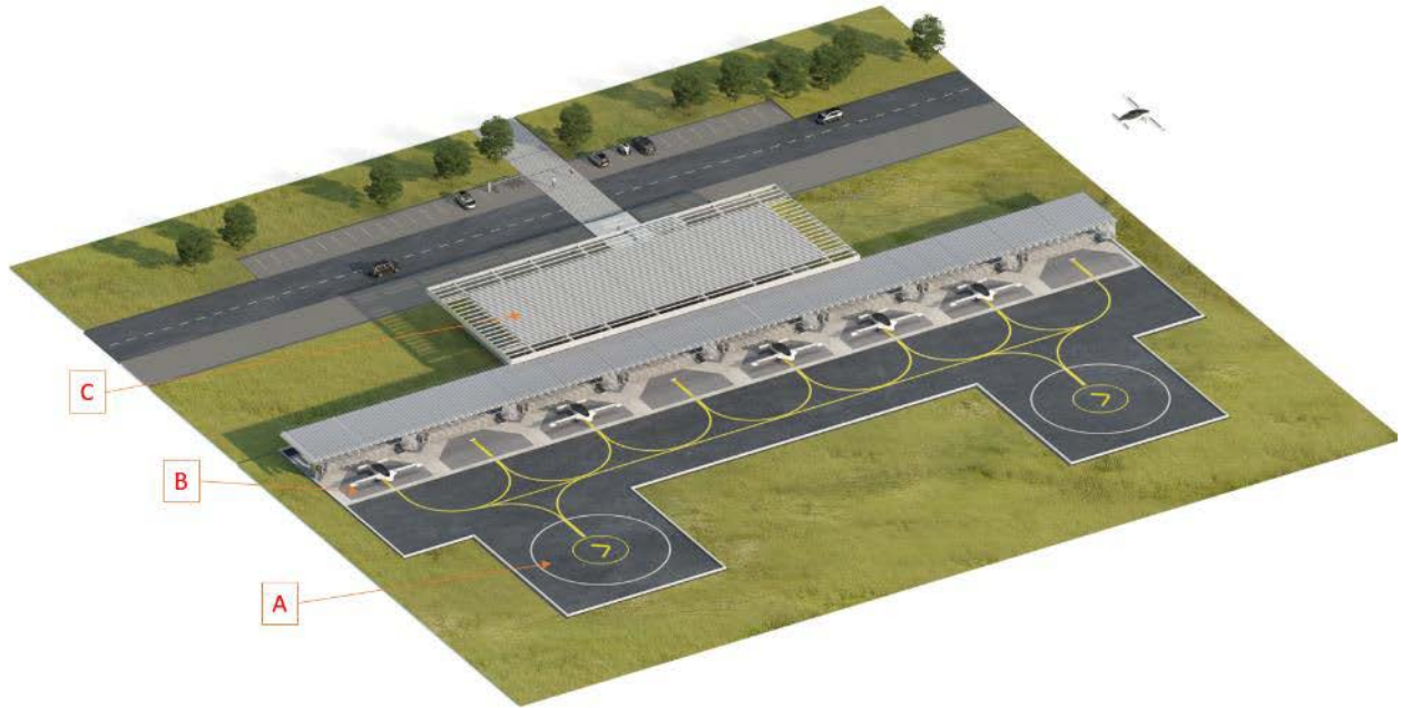
Figure 9. Lilium’s Urban Vertiport Layout with (a) Takeoff Area, (b) Parking Stands, and (c) Terminal
