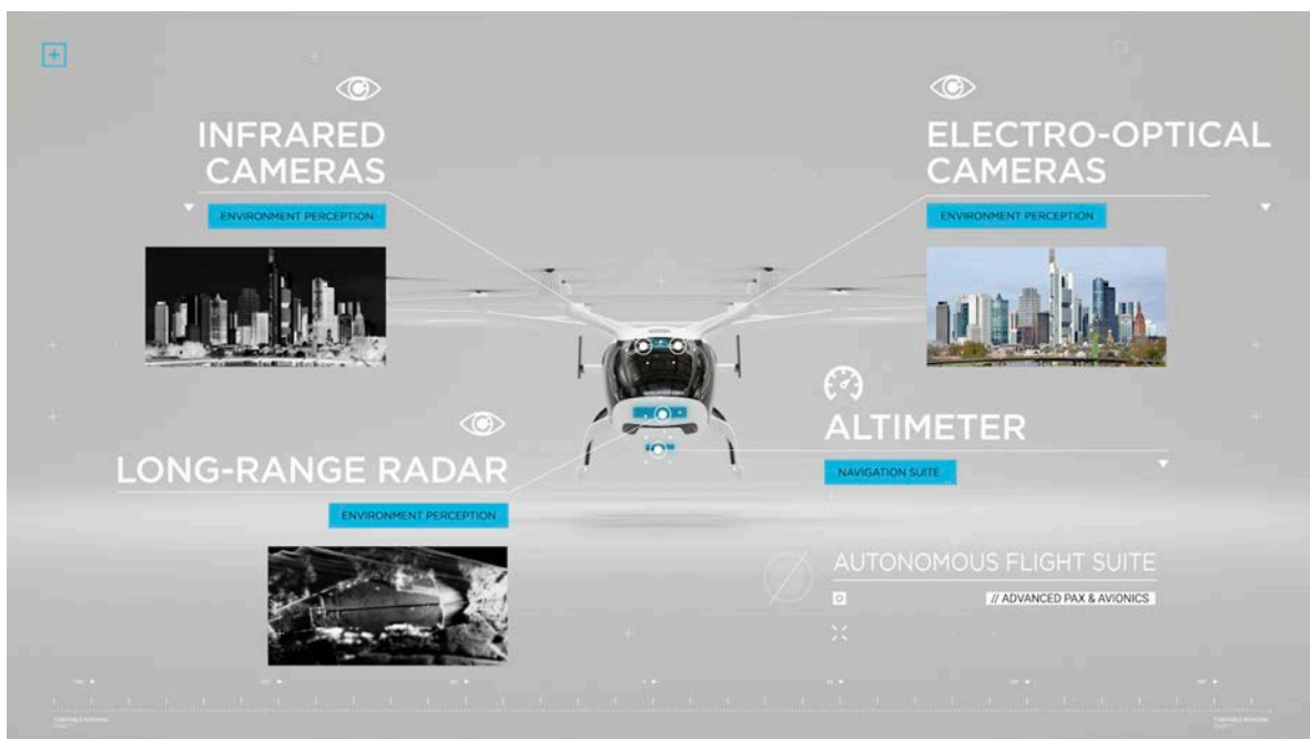
Figure 15 The current Volocity sensor suite captures all information required for autonomous flight.
