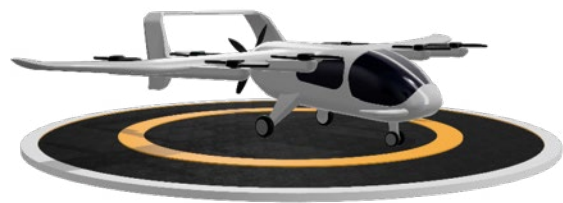
Figure 4: Example of a lift + cruise VCA
