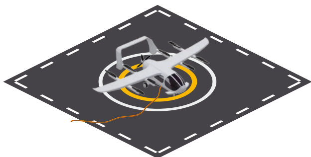
Figure 9: A VCA parked at a vertistop being charged
